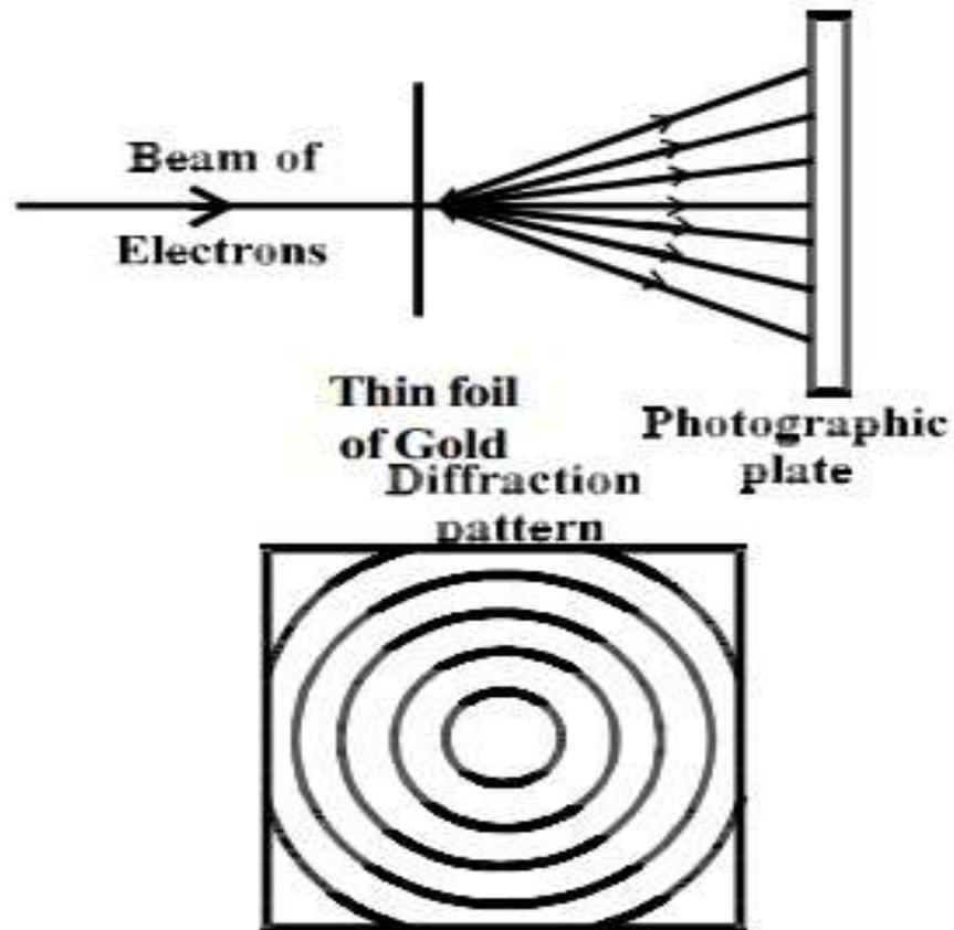
**Diffraction of electron beam by thin foil of gold (G.P. Thomson experiment)**
