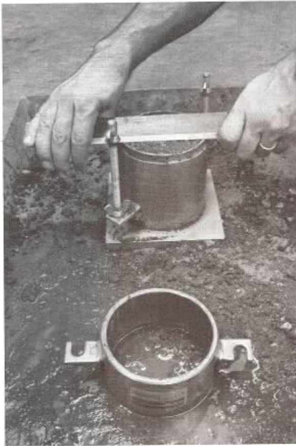
Figure 12.4. Excess soil being trimmed (Step 8).
