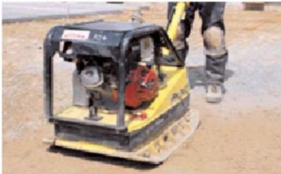
Fig. 11-3. (top) Adequate compaction of a base course foundation for concrete pavement can be achieved by using a vibratory roller. (bottom) Vibratory plate compactors are also used to prepare subgrades under slabs. (69934, 69930)
