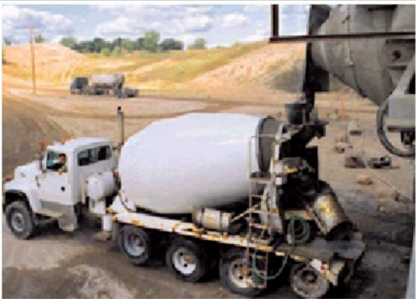
Fig. 10-3. Central mixing in a stationary mixer of the tilting drum type with delivery by a truck mixer operating at agitating speed. (69926)
