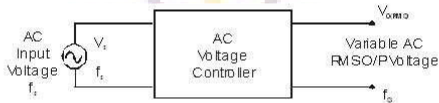
Figure: 3.1 Block diagram of AC voltage controller
