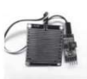
(i) Rainfall sensor
