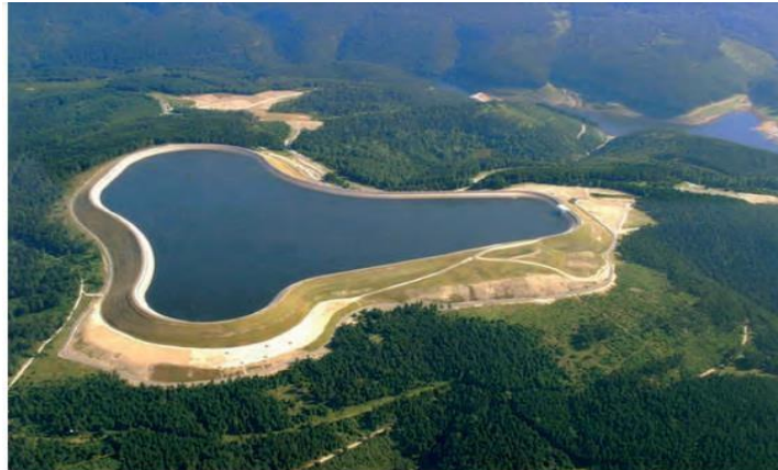
Figure.2.2 Pumped Hydro Storage
