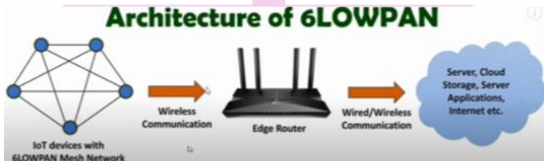
Figure 3.18 : Architecture of 6LoWPAN
