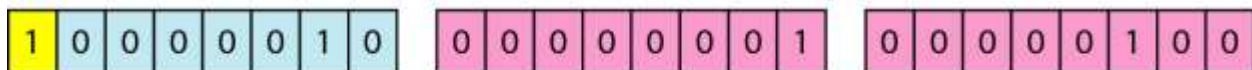
b. The shaded part defines the length of the length (2 bytes); the colored bytes define the length (260 bytes).
