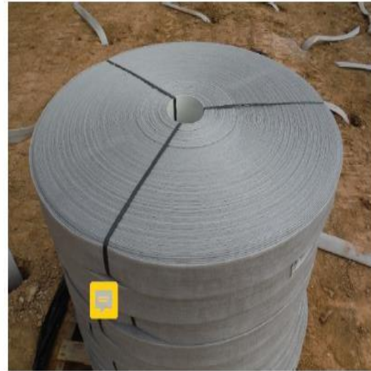
Figure 5. Example of wick drain material rolls.
