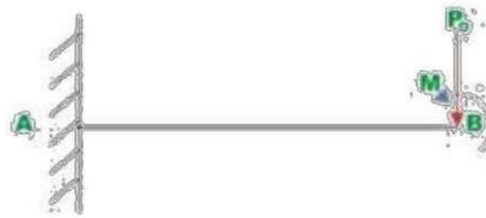
Fig.23.3(a) Cantilever beam
