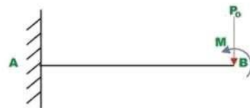
Fig. 23.2(a) Cantilever beam
